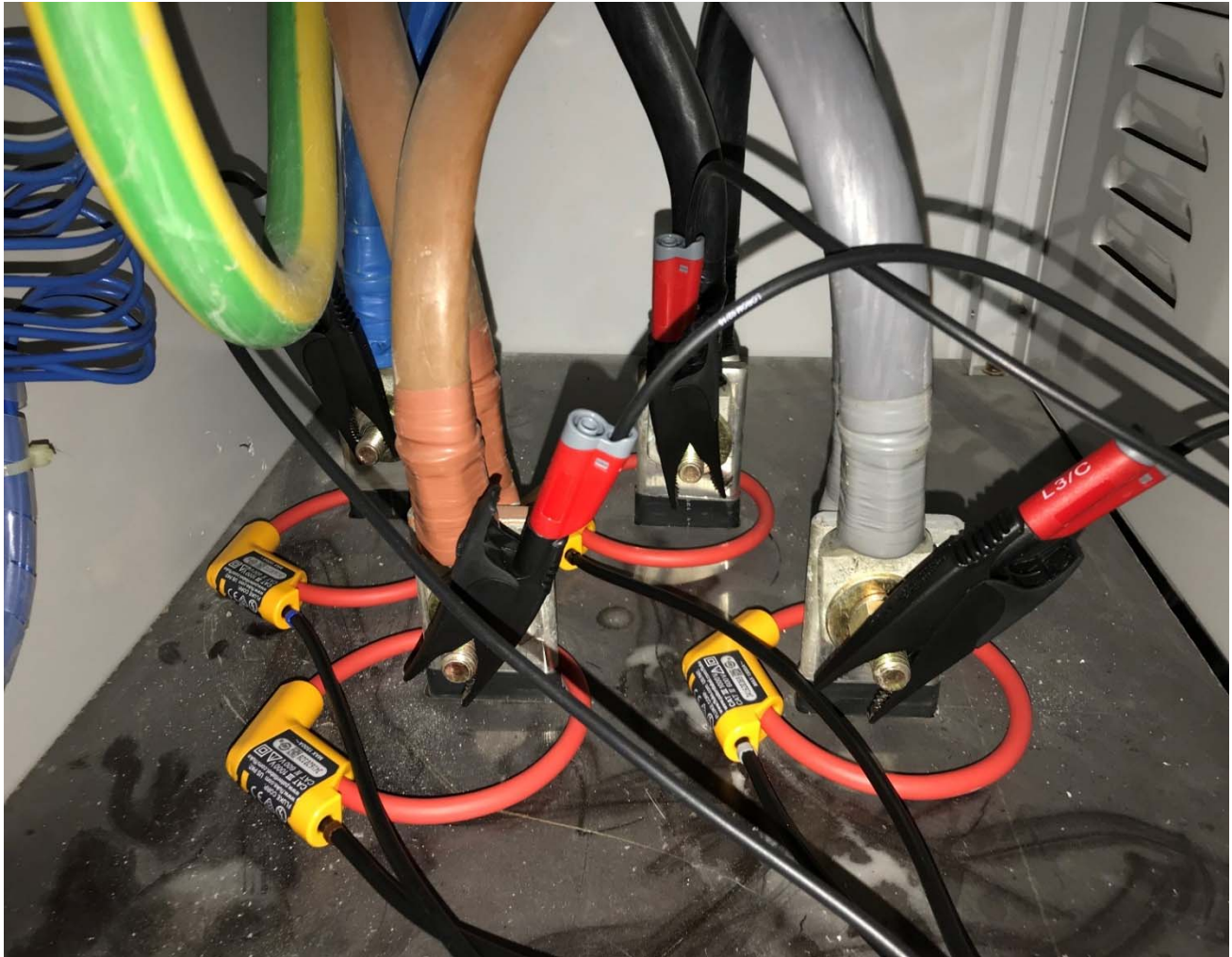
Figure 4.4.2.1 Set Up for Capacitor Bank Measurement
